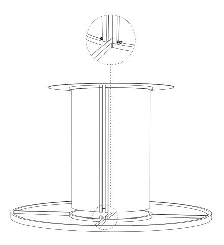
2. Place the table top on a secured surface and turn around the assembled base to fit into the table top frame. Place the screws in position and fasten tight. Repeat on opposite side of the legs.
