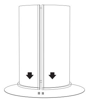
1. Place the bottom plate on a secured surface and fit both legs into the bottom plate. Place the screws in position and fasten tight. Repeat on opposite side of the legs.
