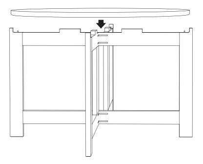
Place the table top on the frame. Make sure that the joints and dowels fit correctly. If needed rotate the table top  $90^\circ$  clockwise until perfect fit.
